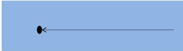
When making a plunge cut, drill a relief hold 1" in diameter near the end of the cut. **IMPORTANT:** *always* cut toward the relief hole.
