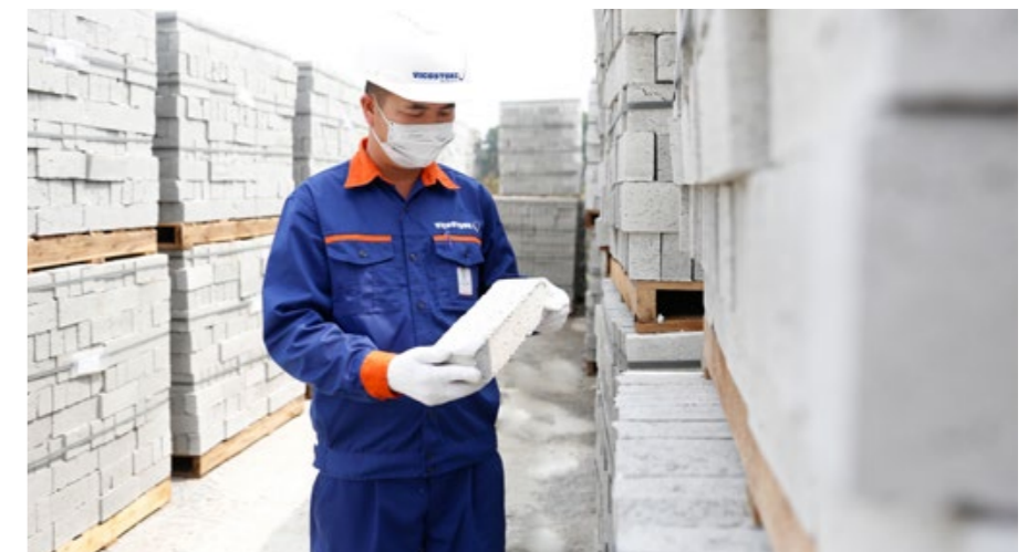
Non-fired bricks made from recycled Vicostone waste stone powder
